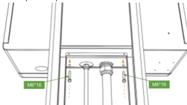
FIG 38: SCHEMATIC DIAGRAM OF MOUNTING HOLE AT THE BOTTOM OF CHARGING BOX
